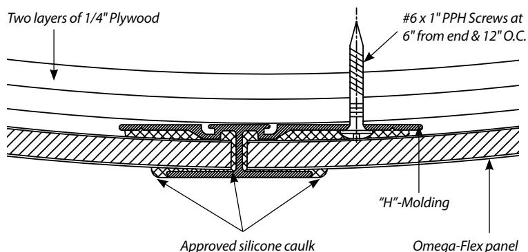
Installation is very similar to flat-panel 1-piece, Tight-Fit molding installation except that glue spacing is reduced to 16" O.C. and no more than 3" from a molding.
