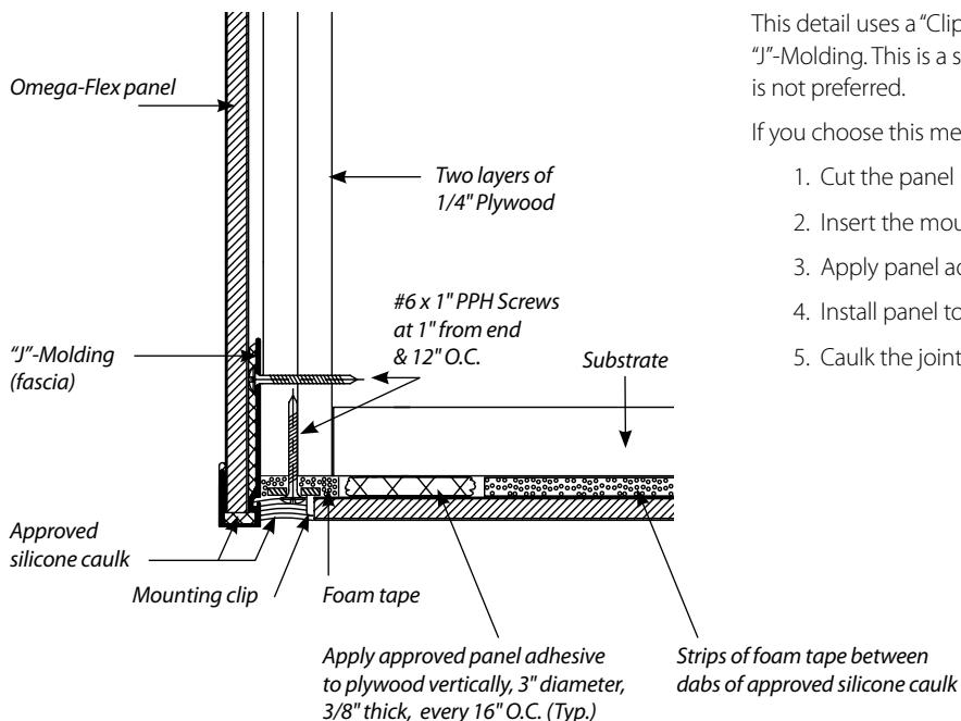
This detail uses a "Clip & Caulk" joint along the soffit, instead of the "J"-Molding. This is a second option that can be used if a "J"-Molding is not preferred.
