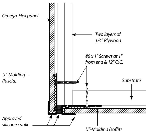
Fascia/Soffit transitions will need to be formed with two "J"-Moldings as shown here, as an outside corner will not conform to a curve. Notice that the fascia molding sits lower than the soffit molding to create a drip edge. This detail can be very difficult on a tight radius. Please call technical support for more information.
