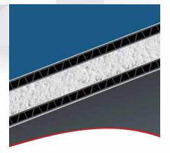
Panels are water-resistant, featuring an insulating core of Polypropolyene (ISO) or Expanded Polystyrene (EPS) foam. Corrugated polypropolyene stabilizers are designed for optimal strength with minimal weight. Prefinished aluminum panels can be ordered in a smooth or stucco-embossed finish in 3/4 in. to 3-1/2 in. overall thickness.
