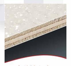
A painted aluminum face bonded to an exterior-grade plywood core to provide an exceptionally strong surface. An aluminum backer completes the panel. Add decorative flair and a very strong and durable surface to fascias, soffits, and storefronts with Omega-Ply architectural panels.
