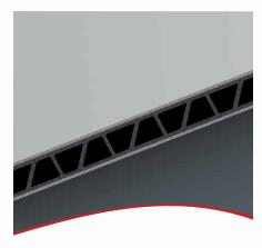
Panels feature a corrugated polypropolyene core for the highest strength-to-weight ratio of any competitive ACM panel. Painted aluminum sheets cover a black, plastic, water-resistant core.
