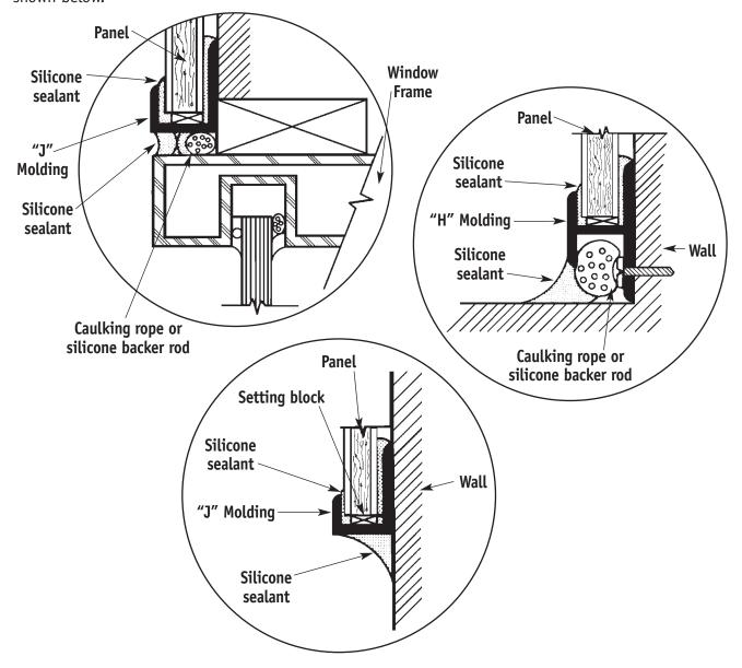
Self-healing sealants should be used at the joints of frame members and glazing stops. Rubber-forming sealants should be used between moldings and adjacent building materials.
