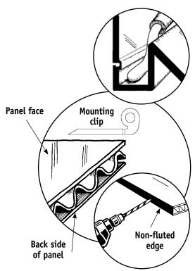
When installing panels with metallic finishes, it is very important that the directional arrows on the panel masking are oriented in the same direction.
