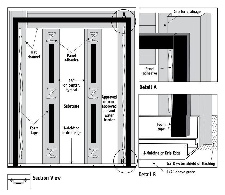
Again, the main drawing depicts the layout for one panel at ground level. As with previous substrates, J-Molding is shown at ground level. Either J-Molding or Drip Edge moldings can be used here. (See 1-Piece, Tight-Fit Installation Guide for complete installation instructions for J- or Drip Edge Moldings.)
