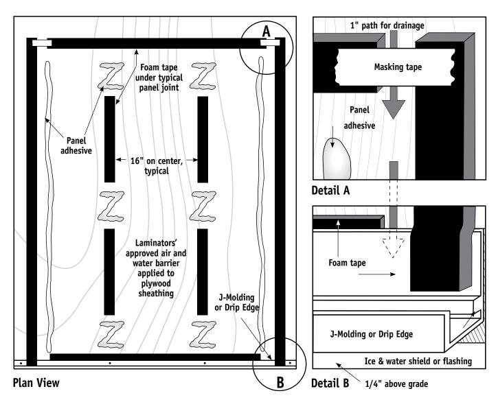
Installation over exterior-grade plywood sheathing with a Laminators' approved, fluid-applied air and water barrier is the base substrate for mounting panels. You should read and understand this process before attempting to mount panels over other substrates.
