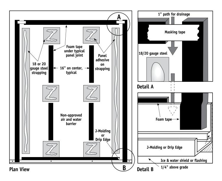
In cases where panels are to be installed over plywood sheathing that is covered with an air and water barrier that has not been pre-approved by Laminators through testing, the following process must be used. Remember, while the plywood sheathing is structural, the compatability of panel adhesive with the non-approved air and water barrier are unknown.
