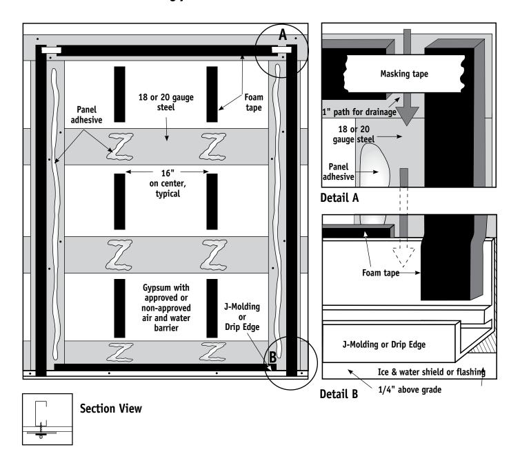
When installing panels over exterior grade gypsum with a Laminators' approved or non-approved air and water barrier, remember that exterior grade gypsum is not structural sheathing.
