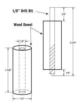
A Clip & Caulk installation with corrugated panels requires drilling and back-venting each panel prior to installation. Carefully follow the steps below to prevent failed caulk joints. Failure to do so may void your warranty.
